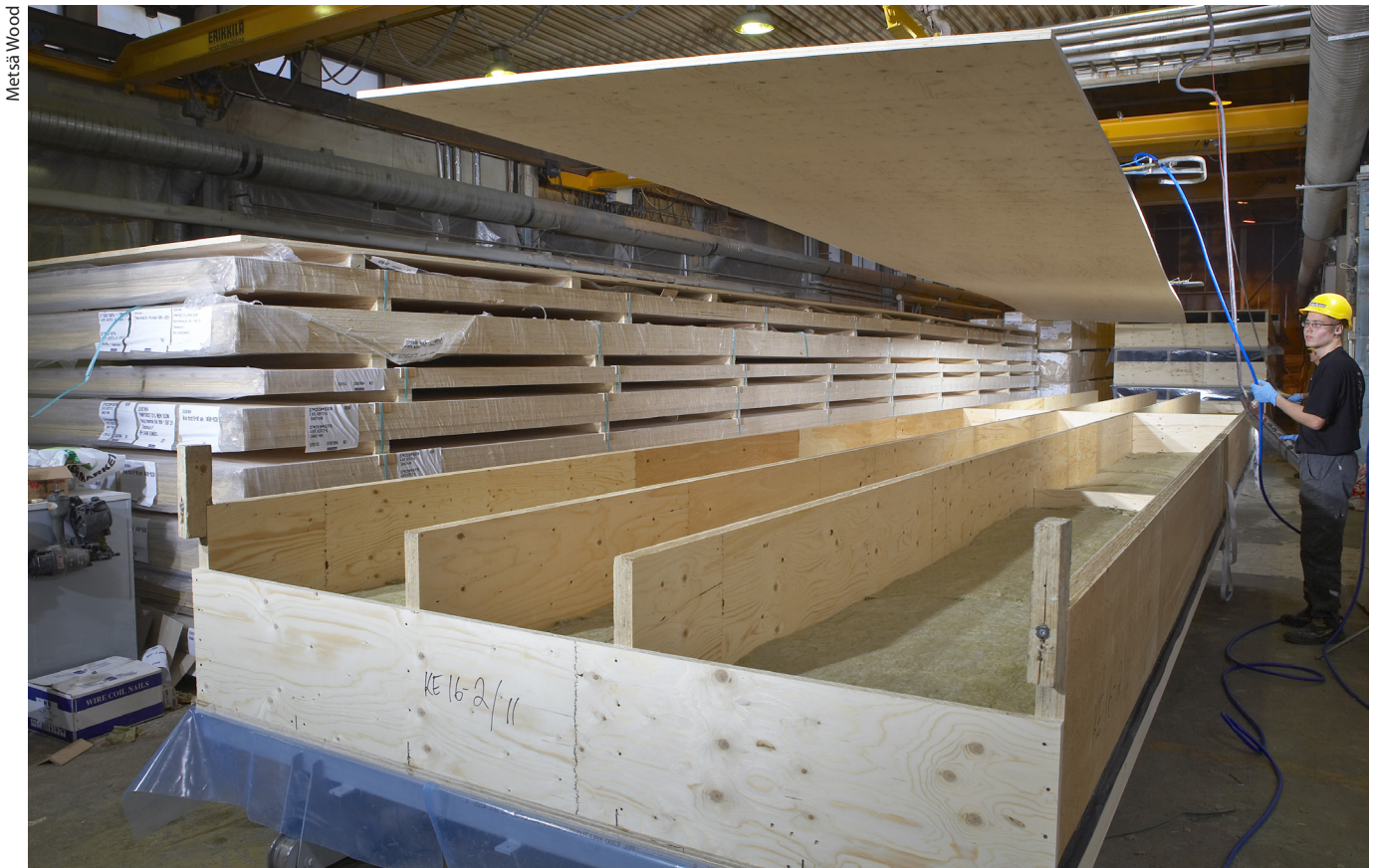
Figure 1.57: Manufacture of structurally glued LVL roof elements.
