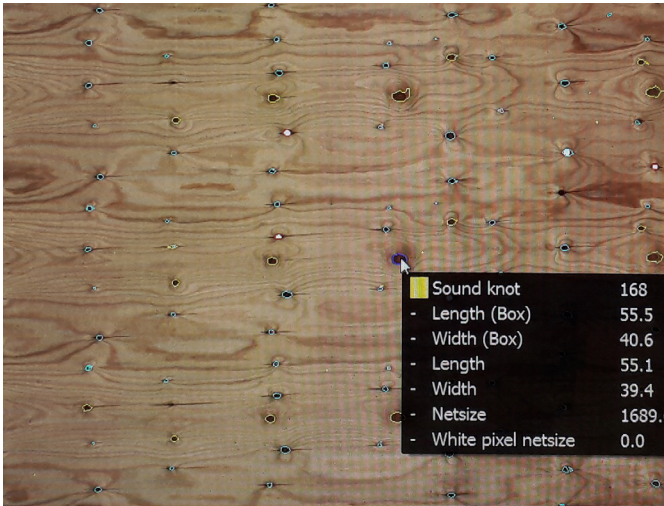
Figure 1.30. VDA camera image for visual defect analysis.
