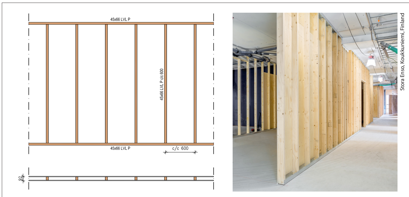
Figure 2.57. LVL-P studs for non-load-bearing interior walls.
