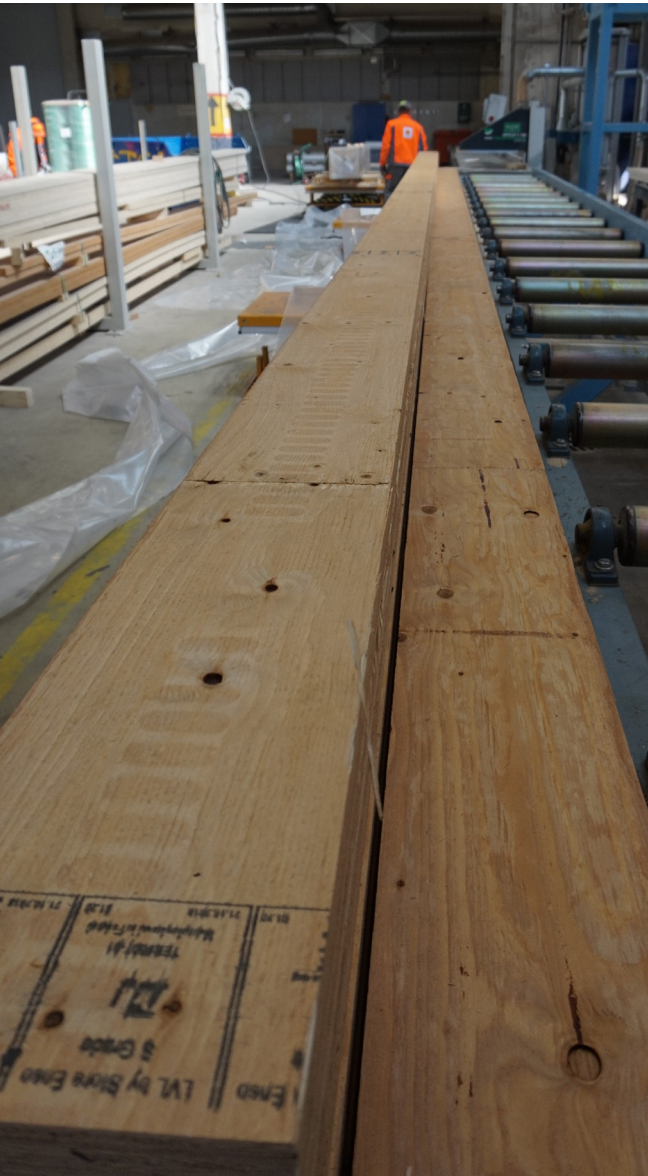
Figure 1.54. Moisture protection treatment of LVL-P beams by Stora Enso.
