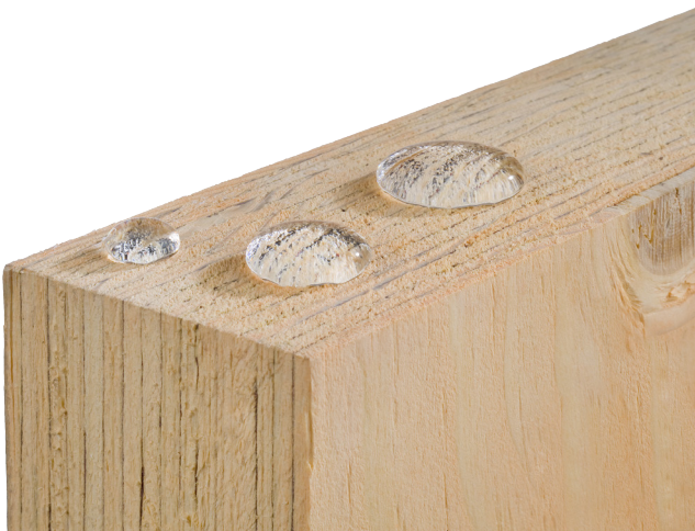
Figure 7.3. Moisture protection treatment on LVL beams.
