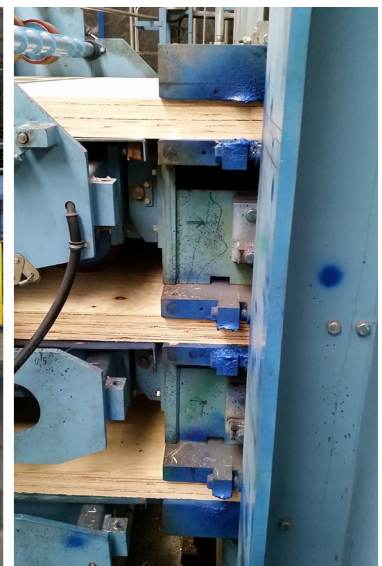
Figure 1.43. Feeding LVL billets into 3-level hot press.
