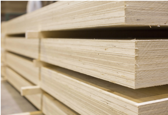
Figure 3.4. Storage of LVL packages
