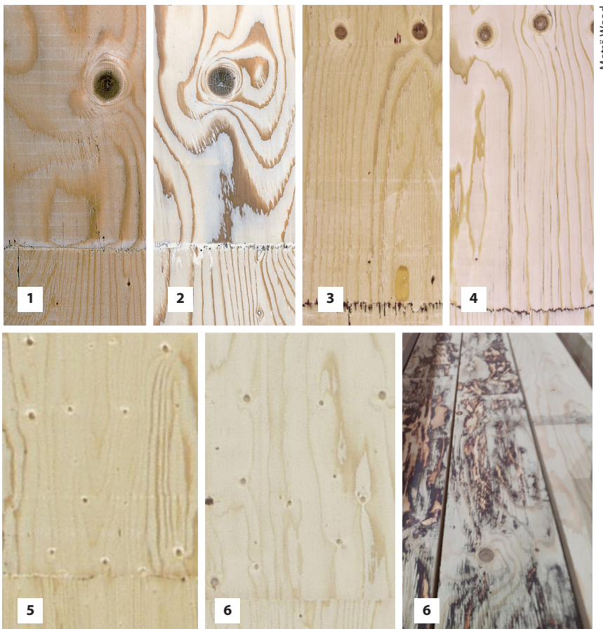
Figure 1.65: Appearance of LVL veneer surfaces 1. Unsanded front side, close image 2. Optical sanded front side, close image 3. Unsanded reverse side with dark scarf-joint glue line, close image 4. Optical sanded reverse side with dark scarf-joint glue line, close image 5. Unsanded front side, general view 6. Optical sanded front side, general view 7. Calibration sanding revealing the dark glue line 11 .
