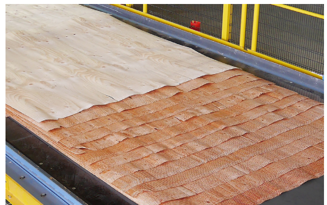
Figure1.40. Staggered layup ahead of the pre-press.
